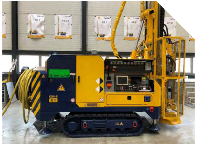
THE DRILLING RIG – KB0-ELECTRIC
